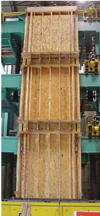
Full-scale test set up for a three-story skipped-floor system.
