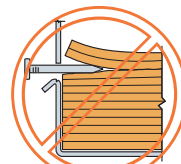
Nail at wrong angle
