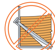
Nail too long
