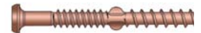
Composi-Lok™ Counterboring Wings and Cap Head Designed to prevent fastener "spin out" with harder materials in cold or wet conditions and "mushrooming" of composite decking material during installation
