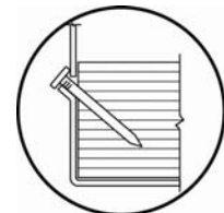
FIGURE 3—POSITIVE ANGLE NAILING (PAN) FOR LBV AND BA SERIES HANGERS
