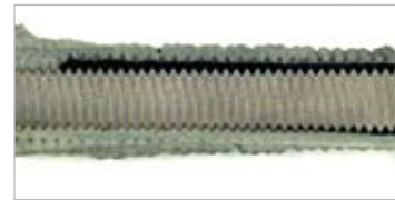
Competitor's screen tube leaves portion of anchor rod unbonded
