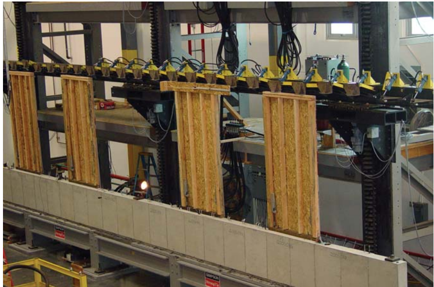
Full-scale shearwall cyclic tests with MAS Anchors at the Tyrell Gilb Laboratory.
