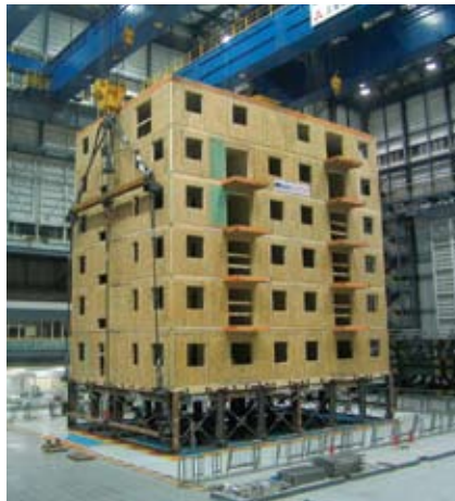
The complete structure weighs 880,000 pounds and it took several hours to move it from the laboratory floor onto the shake table.
