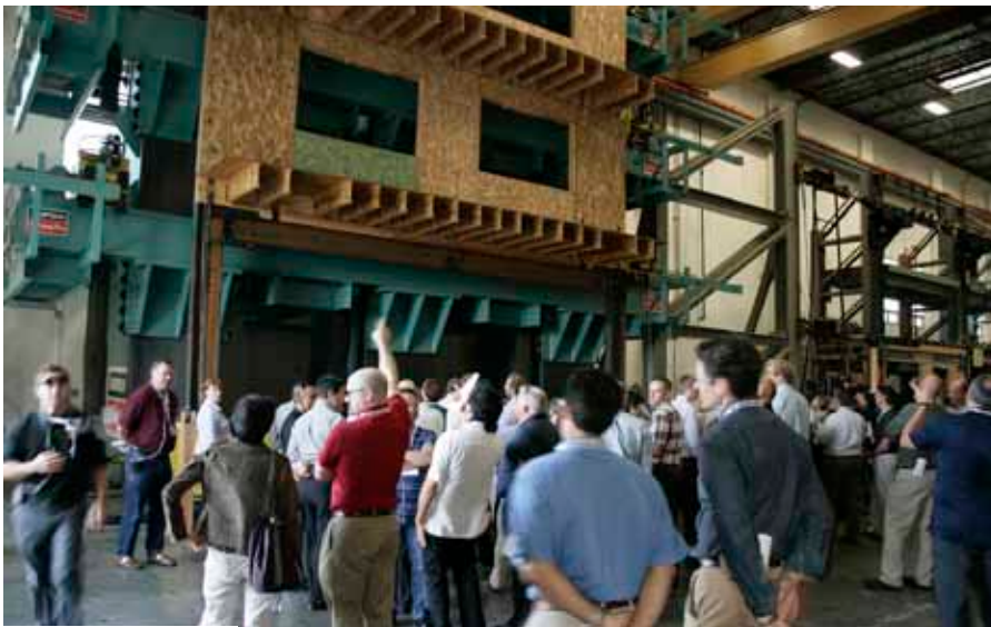
Attendees gathered at the Tye Gilb Lab in Stockton to witness a three-story seismic shake table test.
