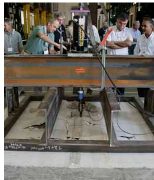
Tension test of a cast-in-place steel anchor rod with plate washer in concrete
