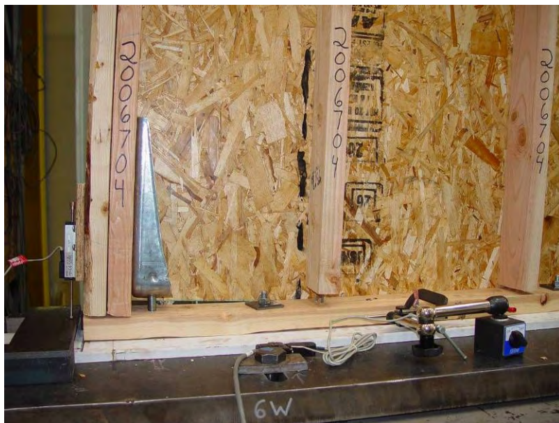
Figure 9 – Typical Deformation after test. <Double corner studs with PhD 5 holddown>
