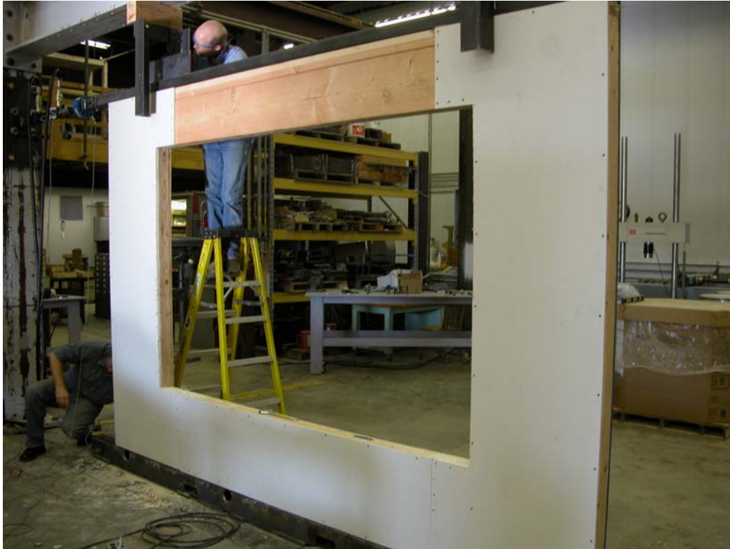
Figure 3. Typical Wall 4_1 Specimen Being Installed in Testing Apparatus Prior to Testing.
