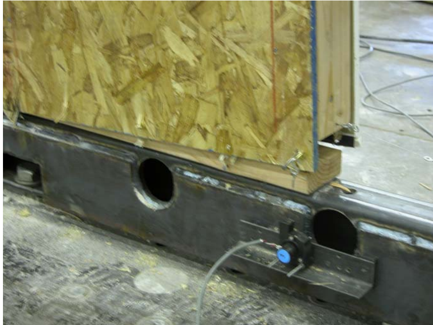
Figure 12. Lifting of Wall Segment from Bottom Plate on 4_1 Wall Specimens.
