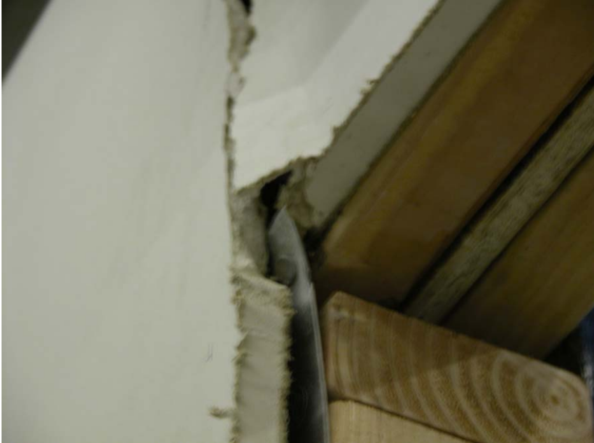
Figure 6. Location of Third Failure in Portal Frame Specimens – Tension Failure of Straps.
